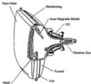
Significant amounts of lead can be found in a CRT’s funnel glass and the frit—the glue that holds together the panel (face plate) and funnel glass of color monitors.
