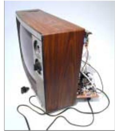
After the electronics were separated into product categories, WM-ARG demanufactured the used products for recyclable materials. Products at the site were generally manually taken apart. Demanufacturing involved disassembling the electronics, removing hazardous materials, sorting them into secondary materials categories and weighing each secondary materials category.
